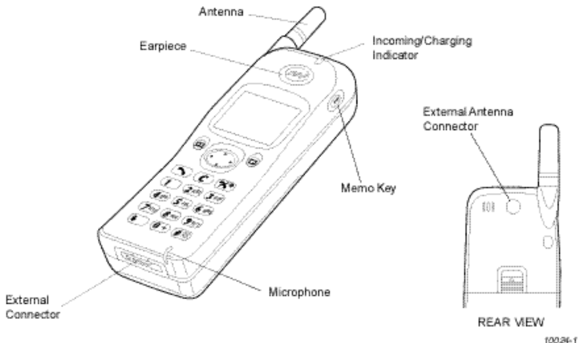
Figure 3.2: Location of controls for GD90
